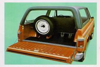
The Jimmy is as wide as a standard pickup and the effective load length behind the drivers seat is 76.6 inches. With the road off there's room for extra bulky objects, and the load length can be extended by dropping the tailgate which is supported by strap-type steel links.
