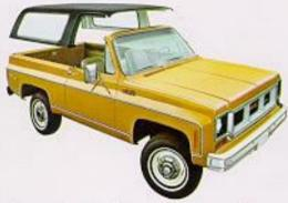
The auxiliary hard top roof with a white or black textured exterior finish and door operated dome light is designed for fast removal and includes a tailgate design with manually operated drop glass. Sliding side glass for the top and tinted glass all around also is available.
