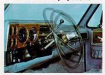
Six-position tilt steering wheel is available with Turbo-Hydra-matic transmissions. Custom 16-inch diameter steering wheel is available in conjunction with power steering.
